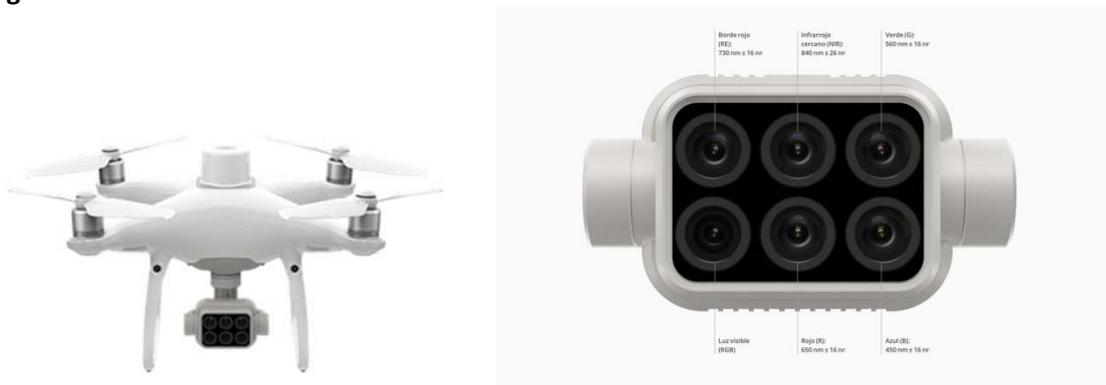
Cámara Multiespectral: RGB, Rojo (650 nm), Azulñ (450 nm), Borde rojo (730 nm), NIR (840 nm) y Verde (560).
