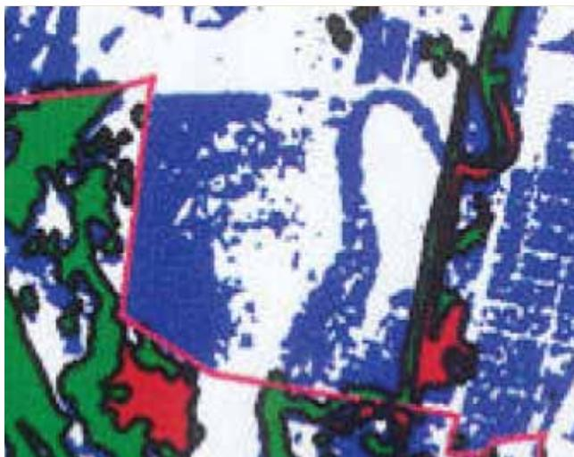
Flooding as shown by a radar image from the RADARSAT satellite (December 1996). The blue shows the levels of flooding in the Caracoles farm in this exceptionally wet year, where the original bed of the Travieso channel is clearly visible. The average maximum flood levels are in green and the minimum levels in red.
