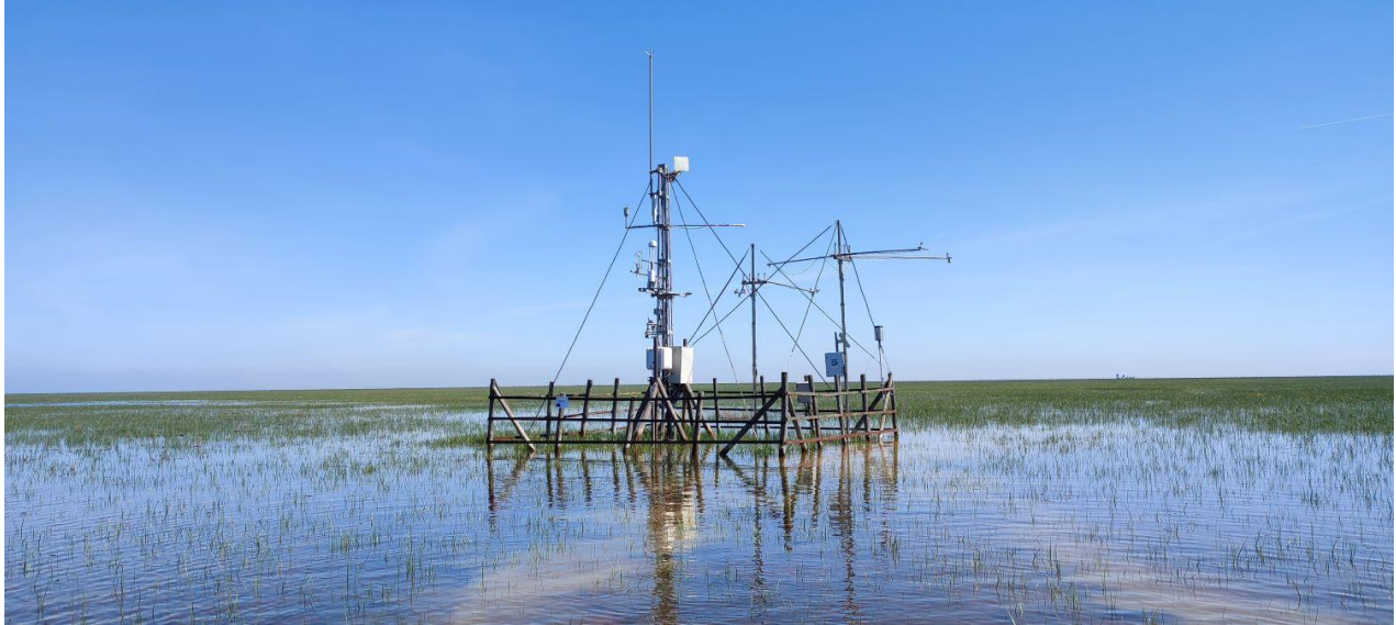
Fuenteduque gas exchange and remote sensing product validation station in the marsh. Photo: Ricardo Díaz-Delgado
